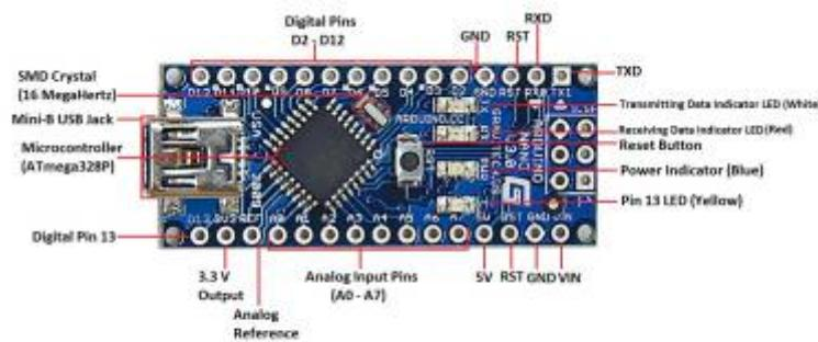
**Arduino Nano V3.0 Pinout**
